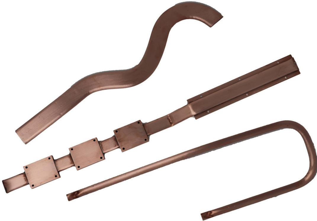
A heat pipe is a heat-transfer device that takes advantage of phase-change properties of the working fluid inside to transfer heat from one end to the other with high efficiency and at a constant temperature gradient.
